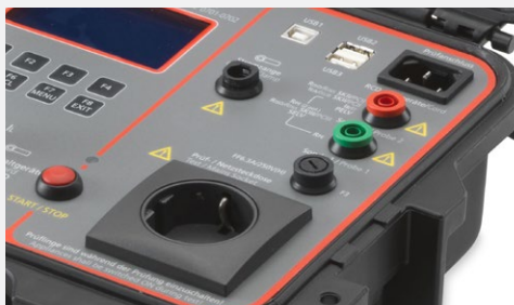
Connection for external current clamp (optional Beha-Amprobe CHB 1) for measuring earth leakage currents, even on 3-phase appliances (GT-900 only).
