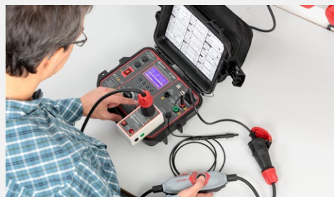
Testing of portable RCDs (PRCD, PRCD-S, PRCD-S+, PRCD-K) (GT-900 only).
